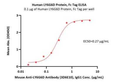
Immobilized Human LY6G6D Protein, Fc Tag (Cat. No. LYD-H5265) at 1  $\mu g/mL$  (100  $\mu L/well)$  can bind Mouse Anti-LY6G6D Antibody (3D6E10), IgG1 with a linear range of 0.02-0.625  $\mu g/mL$  (QC tested).
