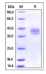
Mouse PD-L2, His Tag on SDS-PAGE under reducing (R) condition. The gel was stained with Coomassie Blue. The purity of the protein is greater than 95%.
