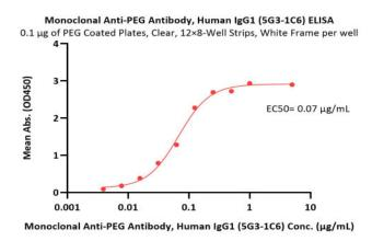
Immobilized PEG Coated Plates, Clear,  $12\times8$ -Well Strips, White Frame at 1  $\mu$ g/mL (100  $\mu$ L/well) can bind Monoclonal Anti-PEG Antibody, Human IgG1 (5G3-1C6) (Cat. No. PEG-M731) with a linear range of 0.004-0.125  $\mu$ g/mL (QC tested).
