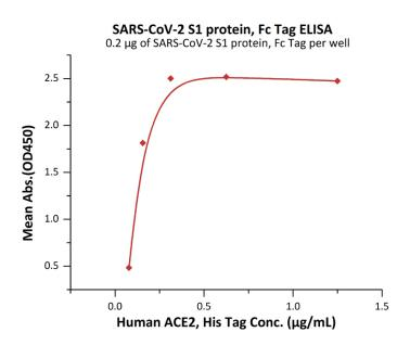
Immobilized SARS-CoV-2 S1 protein, Fc Tag (Cat. No. S1D-C5254) at 2  $\mu$ g/mL (100  $\mu$ L/well) can bind Human ACE2, His Tag (Cat. No. AC2-H52H8) with a linear range of 0.078-0.156  $\mu$ g/mL (Routinely tested).
