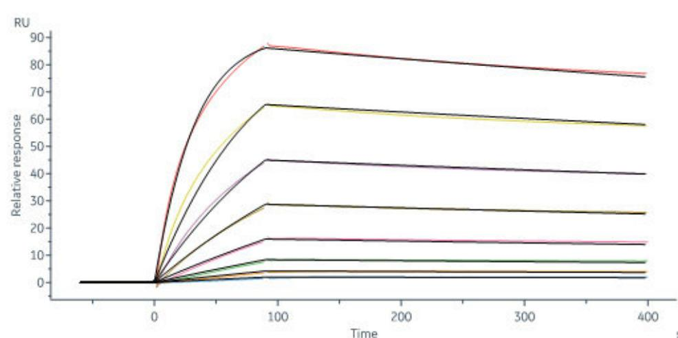
Anti-SEZ6 Antibody (SC17) captured on CM5 chip via anti-Human IgG Fc antibody can bind Human SEZ6 Protein, Mouse IgG1 Fc Tag (Cat. No. SE6-H52F3) with an affinity constant of 6.33 nM as determined in a SPR assay (Biacore 8K) (Routinely tested).
