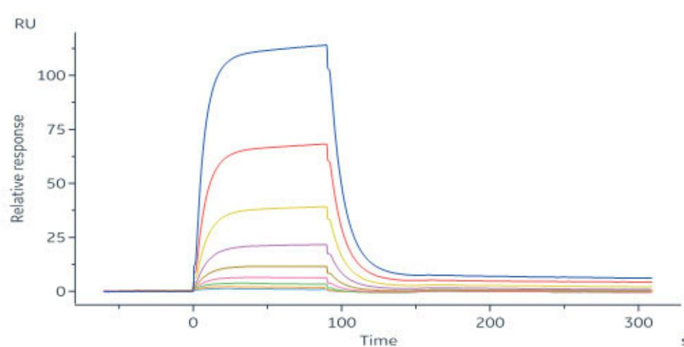
Anti-SEZ6 Antibody (SC17) captured on Protein A Chip can bind Mouse SEZ6 Protein, His Tag (Cat. No. SE6-M52H3) with an affinity constant of 0.947  $\mu$ M as determined in SPR assay (Biacore 8K) (Routinely tested).
