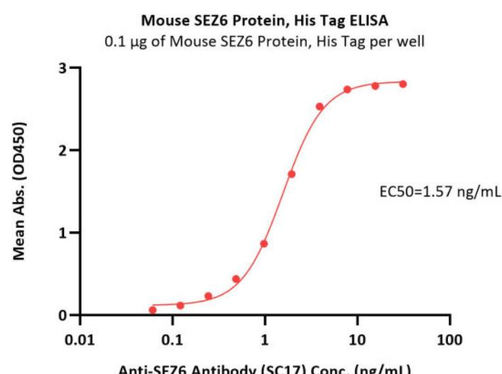
Immobilized Mouse SEZ6 Protein, His Tag (Cat. No. SE6-M52H3) at 1  $\mu$ g/mL (100  $\mu$ L/well) can bind Anti-SEZ6 Antibody (SC17) with a linear range of 0.06-4 ng/mL (QC tested).
