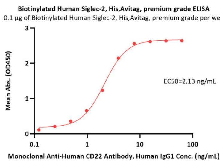
Immobilized Biotinylated Human Siglec-2, His,Avitag, premium grade (Cat. No. SI2-H82E3) at 1  $\mu$ g/mL (100  $\mu$ L/well) on streptavidin (Cat. No. STN-N5116) precoated (0.5  $\mu$ g/well) plate can bind Monoclonal Anti-Human CD22 Antibody, Human IgG1 with a linear range of 0.1-4 ng/mL (QC tested).
