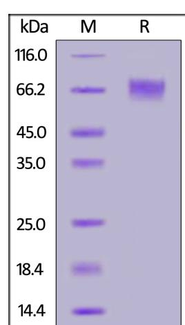
Biotinylated Human Siglec-9, His,Avitag on SDS-PAGE under reducing (R) condition. The gel was stained with Coomassie Blue. The purity of the protein is greater than 95%.
