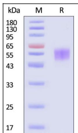
SARS-CoV-2 Spike NTD Protein, His Tag (BA.4 & BA.5/Omicron) on SDS-PAGE under reducing (R) condition. The gel was stained with Coomassie Blue. The purity of the protein is greater than 90% (With [Star Ribbon Pre-stained Protein Marker](#)).
