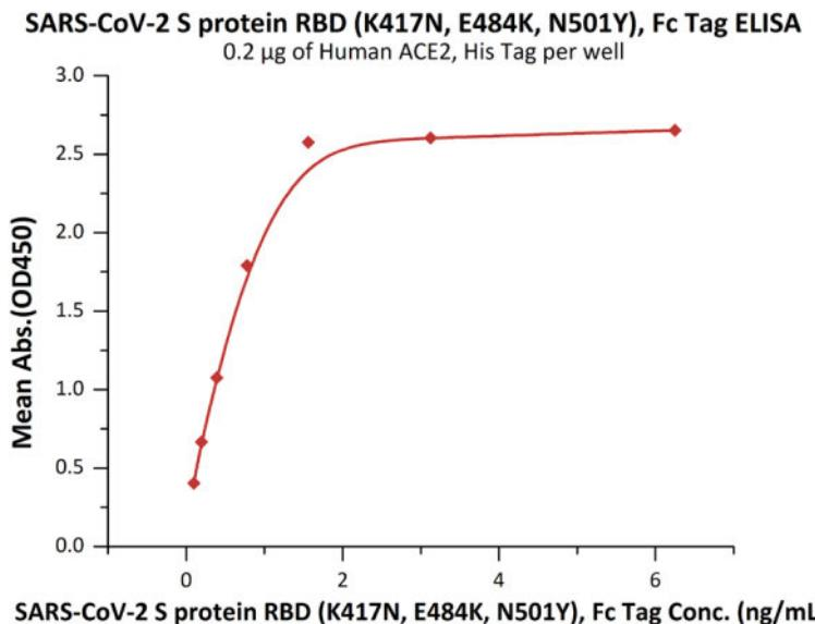
Immobilized Human ACE2, His Tag (Cat. No. AC2-H52H8) at 2 µg/mL (100 µL/well) can bind SARS-CoV-2 S protein RBD (K417N, E484K, N501Y), Fc Tag (Cat. No. SPD-C5256) with a linear range of 0.1-0.8 ng/mL (Routinely tested).
