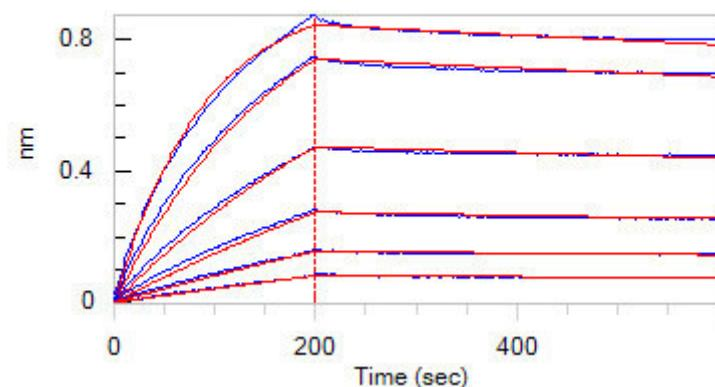
Loaded SARS-CoV-2 S protein RBD, Fc Tag (Cat. No. SPD-C5256) on Protein A Biosensor, can bind Human ACE2, His Tag (Cat. No. AC2-H52H8) with an affinity constant of 2.03 nM as determined in BLI assay (ForteBio Octet Red96e)(Routinely tested).
