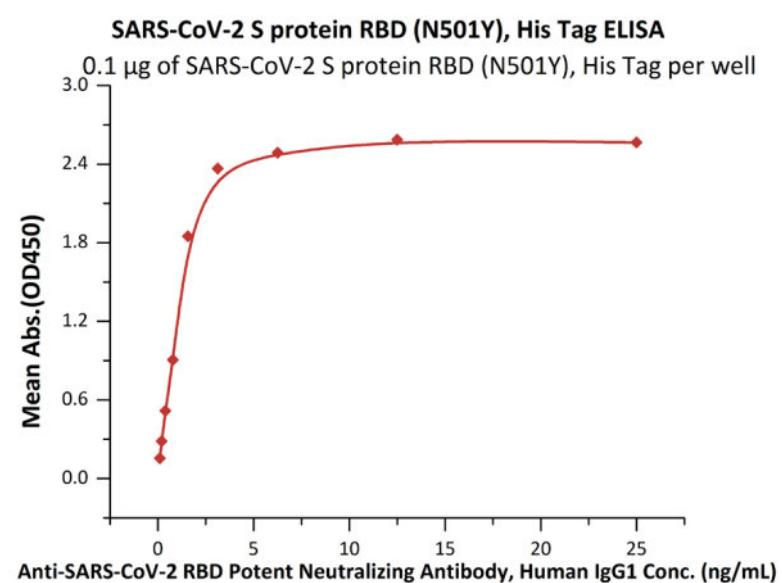
Immobilized SARS-CoV-2 S protein RBD (N501Y), His Tag (Cat. No. SPD-C52Hn) at 1  $\mu$ g/mL (100  $\mu$ L/well) can bind Anti-SARS-CoV-2 RBD Potent Neutralizing Antibody, Human IgG1 (Cat. No. SPD-M180) with a linear range of 0.1-3 ng/mL (Routinely tested).
