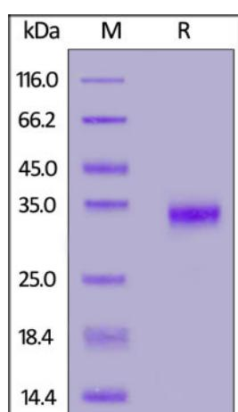
Biotinylated SARS-CoV-2 S protein RBD, His,Avitag on SDS-PAGE under reducing (R) condition. The gel was stained with Coomassie Blue. The purity of the protein is greater than 95%.
