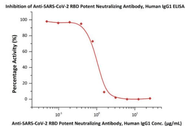
Immobilized SARS-CoV-2 S protein RBD, His Tag (Cat. No. SPD-C52H3) at 1 µg/mL (100 µL/well) can bind Anti-SARS-CoV-2 RBD Potent Neutralizing Antibody, Human IgG1 (AM180) (Cat. No. SPD-M180) with a linear range of 0.2-2 ng/mL (QC tested).
