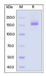
SARS-CoV-2 Spike Trimer, His Tag (BA.3/Omicron) on SDS-PAGE under reducing (R) condition. The gel was stained with Coomassie Blue. The purity of the protein is greater than 95%.
