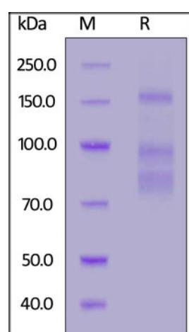
SARS-CoV-2 S protein, His Tag on SDS-PAGE under reducing (R) condition. The gel was stained with Coomassie Blue. The purity of the protein is greater than 95%.
