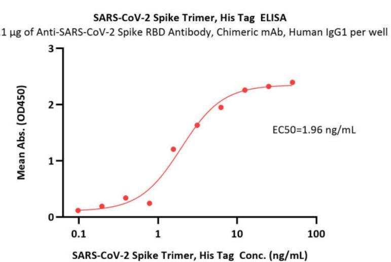
Immobilized Anti-SARS-CoV-2 Spike RBD Antibody, Chimeric mAb, Human IgG1 (Cat. No. S1N-M122) at 1 µg/mL (100 µL/well) can bind SARS-CoV-2 Spike Trimer, His Tag (Cat. No. SPN-C52Hs) with a linear range of 0.1-6 ng/mL (Routinely tested).
