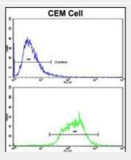
Flow cytometric analysis of CEM cells using ND5 Antibody (C-term)(bottom histogram) compared to a negative control cell (top histogram). FITC-conjugated goat-anti-rabbit secondary antibodies were used for the analysis.
