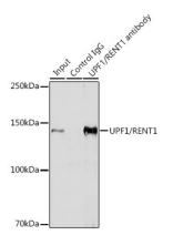
Immunoprecipitation analysis of 300  $\mu$ g extracts of HeLa cells using 3  $\mu$ g UPF1/RENT1 Rabbit mAb(A5071). Western blot was performed from the immunoprecipitate using UPF1/RENT1 Rabbit mAb(A5071) at a dilution of 1:1000.
