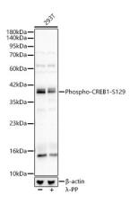
Western blot analysis of lysates from 293T cells, using Phospho-CREB1-S129 Rabbit pAb (AP1437) at 1:400 dilution. 293T cells were treated by  $\lambda$ -PP mixed solution (1ul) at 30°C for 30 minutes.
