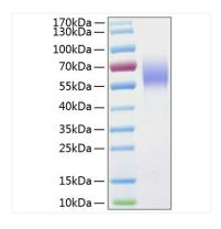
Recombinant Human IL-13RA1/CD213a1 Protein was determined by SDS-PAGE with Coomassie Blue, showing a band at 55-70 kDa.
