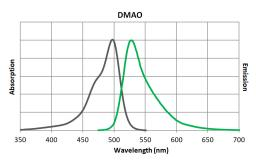
Figure 1. Normalized absorption and emission of DMAO.
