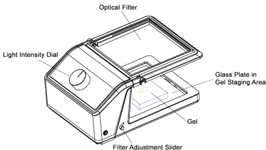
Figure 3. Diagram of Gel-Bright™ Laser Diode Gel Illuminator.
