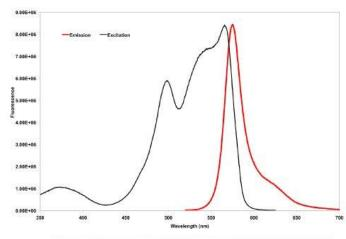
Fluorescence excitation and emission spectra of R-phycoerythrin in 100 mM sodium phosphate (pH 7.2) + 1 mM EDTA and 1 mM sodium azide. Emission scan was taken with excitation at 498 nm. Excitation scan was taken with emission at 575 nm. Scans were normalized to equalize peak heights.
