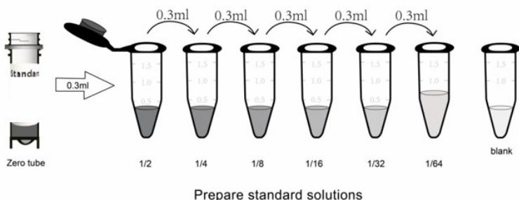
**Notes:** Store the zero tube with dissolved standards at 2-8°C. Other diluted working solutions containing standards should be used in 2h.
