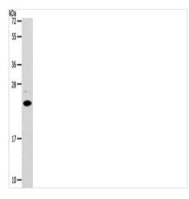
Gel: 12%SDS-PAGE, Lysate: 40 µg, Lane: Mouse liver tissue, Primary antibody: CSB-PA187305(SOD2 Antibody) at dilution 1/950, Secondary antibody: Goat anti rabbit IgG at 1/8000 dilution, Exposure time: 30 seconds
