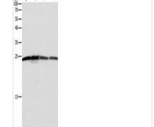
Gel: 12%SDS-PAGE, Lysate: 40 µg, Lane 1-4: Hela cells, A431 cells, 293T cells, Jurkat cells, Primary antibody: CSB-PA299203(BAK1 Antibody) at dilution 1/550, Secondary antibody: Goat anti rabbit IgG at 1/8000 dilution, Exposure time: 5 seconds
