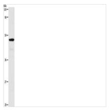
Gel: 10%SDS-PAGE, Lysate: 30 μg, Lane: HepG2 cells, Primary antibody: CSB-PA808693(SERPINA3 Antibody) at dilution 1/250, Secondary antibody: Goat anti rabbit IgG at 1/8000 dilution, Exposure time: 30 seconds
