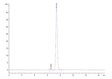
The purity of Biotinylated Human PTK7 is greater than 95% as determined by SEC-HPLC.
