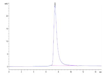
The purity of Mouse CD38 is greater than 95% as determined by SEC-HPLC.
