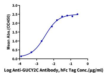
Immobilized Biotinylated Human GUCY2C, His-Avi Tag at 0.5µg/ml (100µl/Well) on streptavidin (5µg/ml) precoated plate. Dose response curve for Anti-GUCY2C Antibody, hFc Tag with the EC50 of 3.1ng/ml determined by ELISA.
