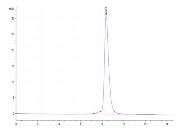
The purity of Biotinylated Human GUCY2C is greater than 95% as determined by SEC-HPLC.
