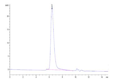
The purity of Human IL-15RA is greater than 95% as determined by SEC-HPLC.
