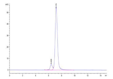
The purity of Cynomolgus LY75 is greater than 90% as determined by SEC-HPLC.
