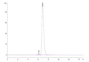
The purity of Human HLA-A\*03:01&B2M&gp100 (ALLAVGATK) Tetramer is greater than 95% as determined by SEC-HPLC.
