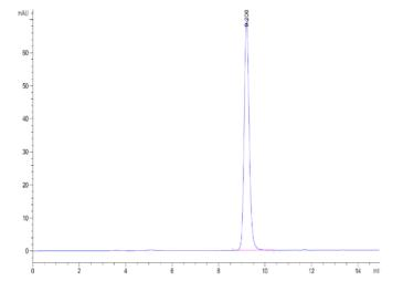
The purity of Biotinylated Human HLA-E\*01:03&B2M&EBV LMP1 (GGDPHLPTL) Monomer is greater than 95% as determined by SEC-HPLC.
