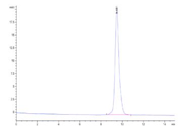
The purity of Human MSLN is greater than 95% as determined by SEC-HPLC.
