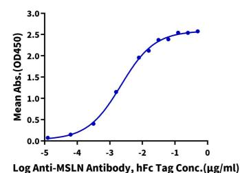
Immobilized Human MSLN, His Tag at 1µg/ml (100µl/well) on the plate. Dose response curve for Anti-MSLN Antibody, hFc Tag with the EC50 of 2.2ng/ml determined by ELISA (QC Test).
