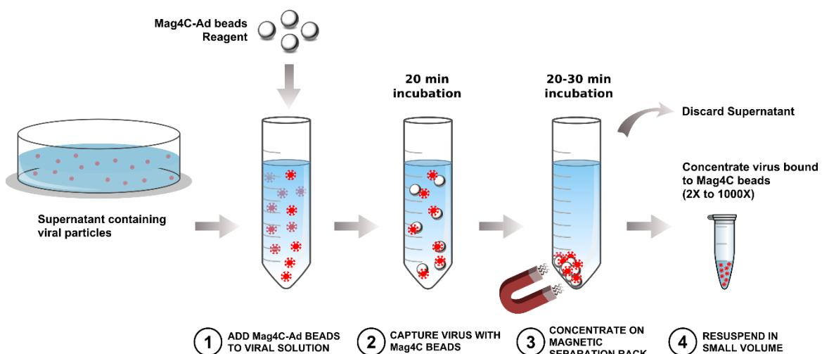
The protocol is simple: 20  $\mu$ L of **Mag4C-Ad** beads are sufficient to bind  $1 \times 10^6$  infectious viruses with almost 80-99% efficiency. Please refer to the **Table 1** for the suggested **Mag4C-Ad** beads volume according to the virus titer.
