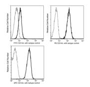
Flow cytometric analysis of Human CD144 expression on HUVEC cells. Cells were stained with PE-conjugated anti-Human CD144. The fluorescence histograms were derived from gated events with the forward and side light-scatter characteristics of intact cells.
