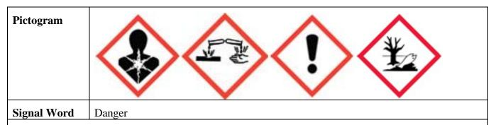
**Hazard Statements:** Harmful if swallowed (H302), Causes serious eye damage (H318), Suspected of causing cancer (H351), Very toxic to aquatic life with long lasting effects (H410).
