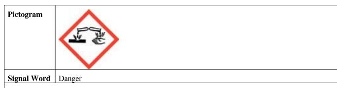
**Hazard Statements:** May be corrosive to metals (H290), Causes severe skin burns and eye damage (H314).
